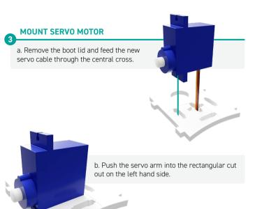
c. Place the boot lid back into its original place, slotting the servo axle through the side panel.
